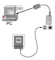
2. Once successfully connected, do a power cycle (unplug and then plug in the power connector) of the NetPort while the HyperTerminal connection is active. As soon as it is ON, press 'xxx' quickly within 3 seconds of connection. You will get the following dialog.
